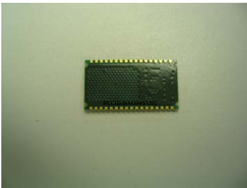
BlueTooth Module inside Bottom View
