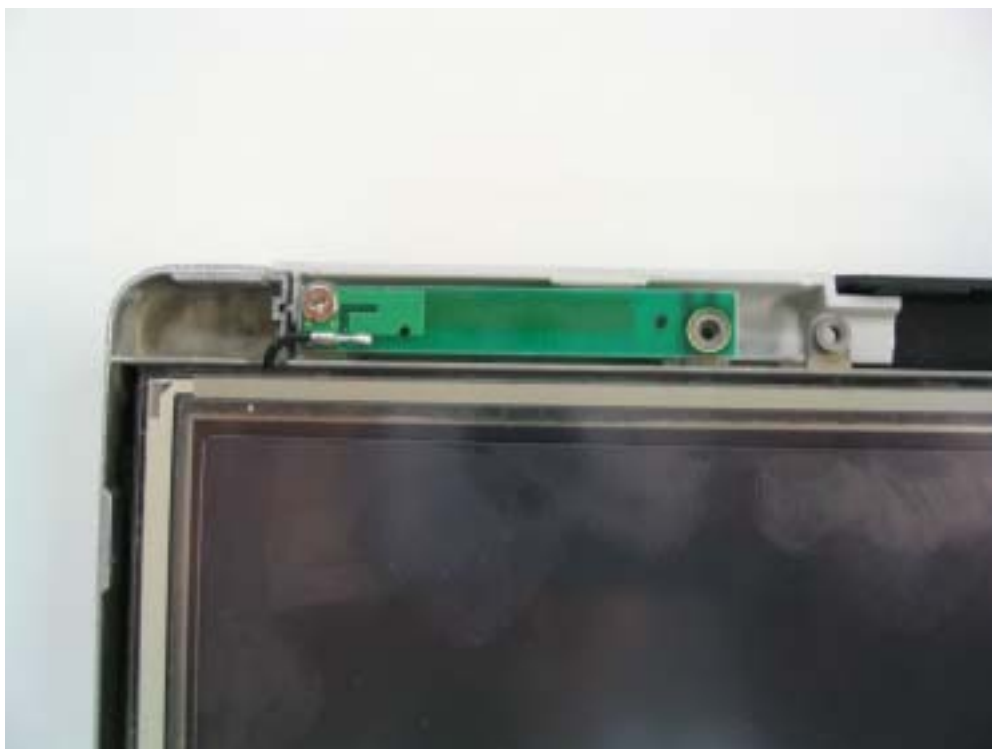
WLAN Main antenna magnified view
