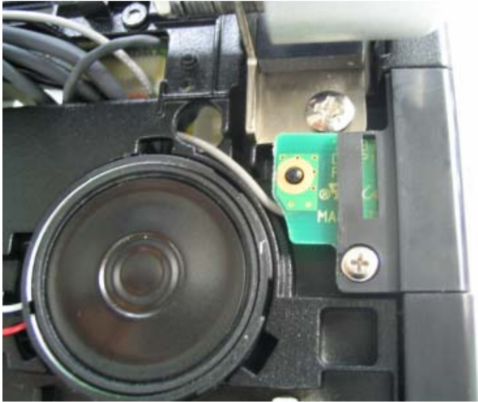
BlueTooth Antenna Magnified View
