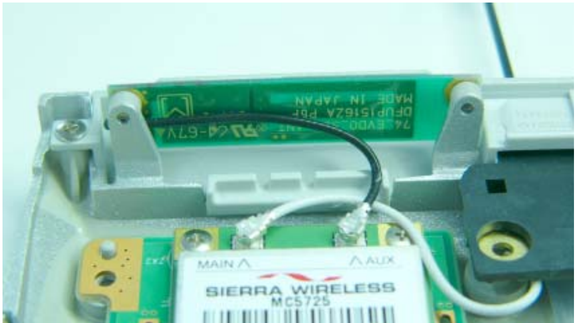
EVDO Aux antenna magnified view
