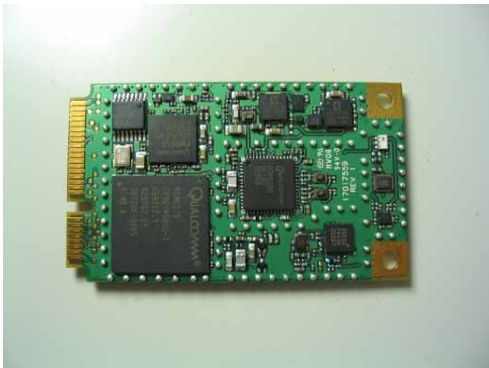
HSDPA Module Interior Bottom View
