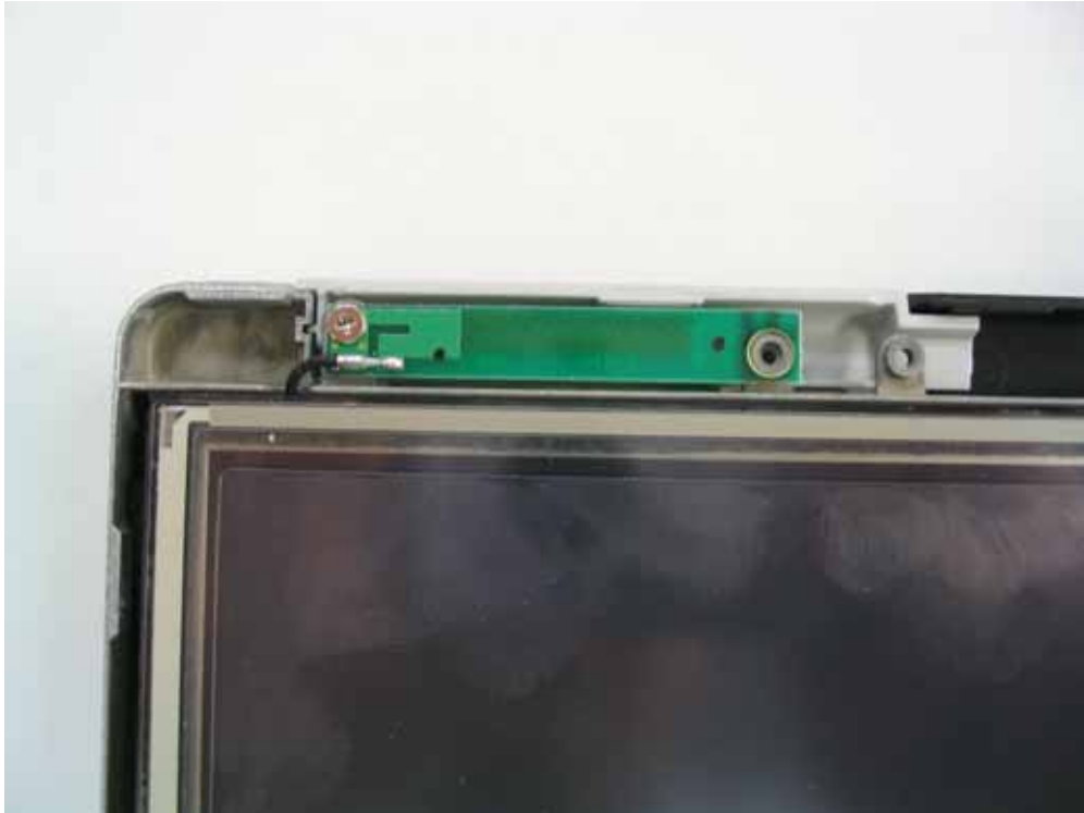
WLAN Main antenna magnified view
