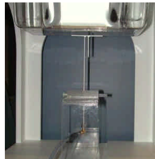
Figure 10.1 Dipole Validation Test Setup
