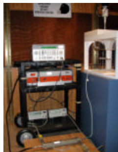
Figure A.0 Dipole Validation Test Setup
