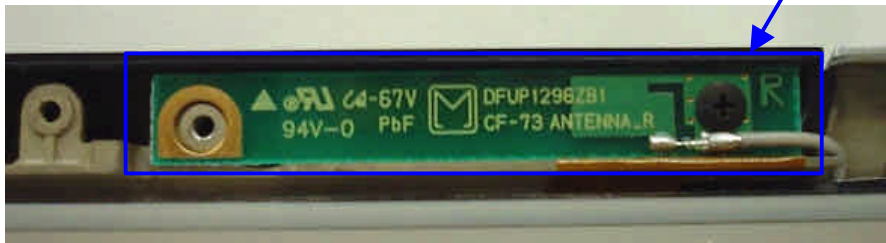
Send & Receive Antenna View
