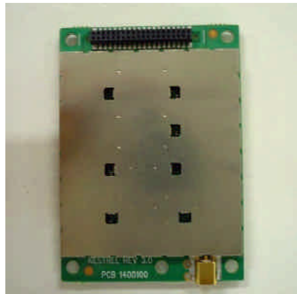
SB555 module Bottom View
