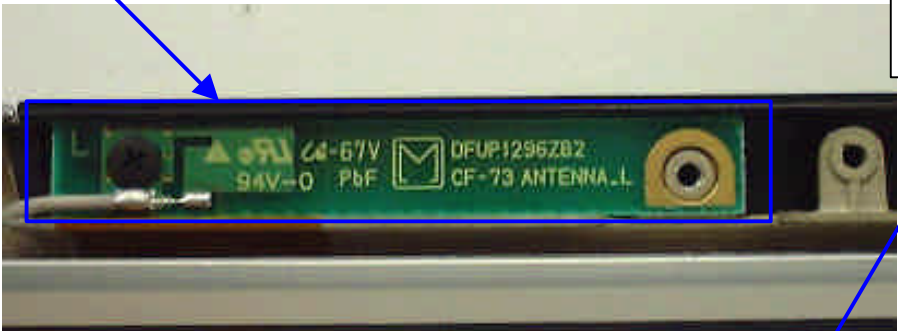
Receive only Antenna View
