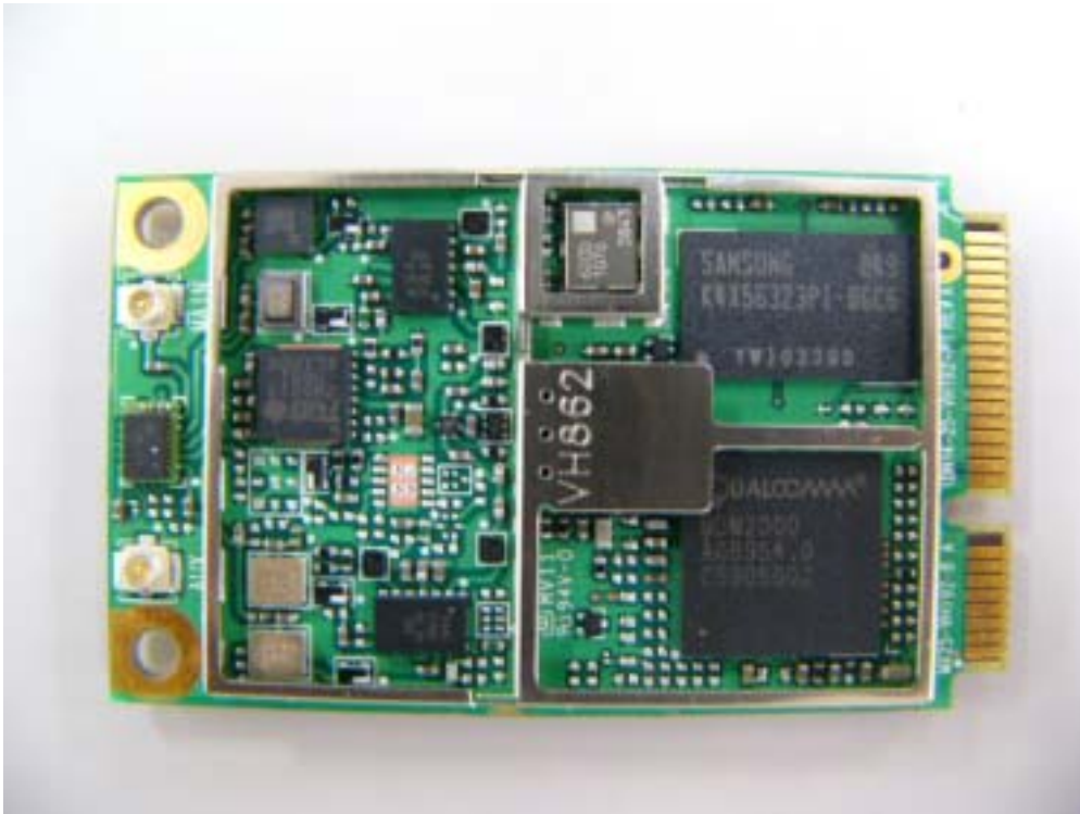
WWAN Module Interior Top View
