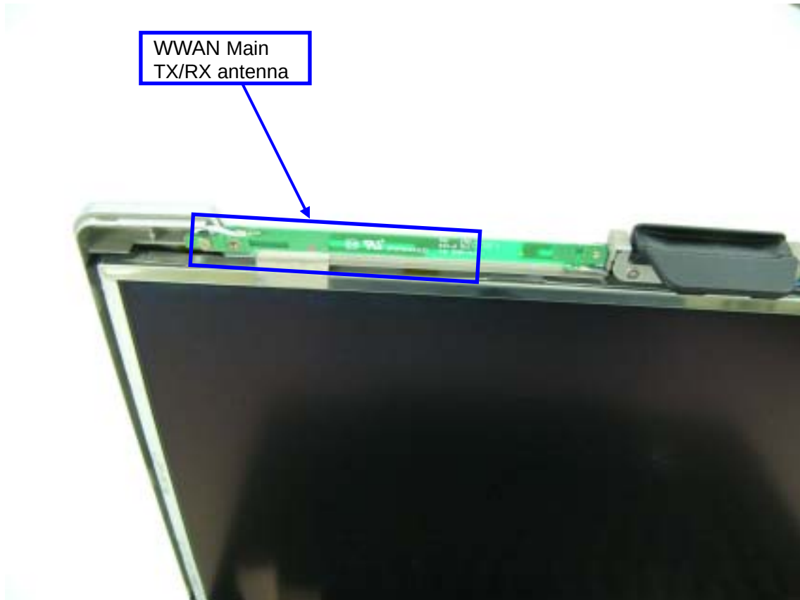
WWAN Main TX/RX Antenna
