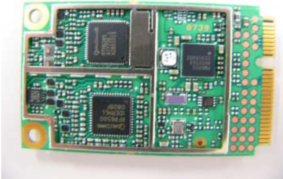
WWAN Module Interior Bottom View
