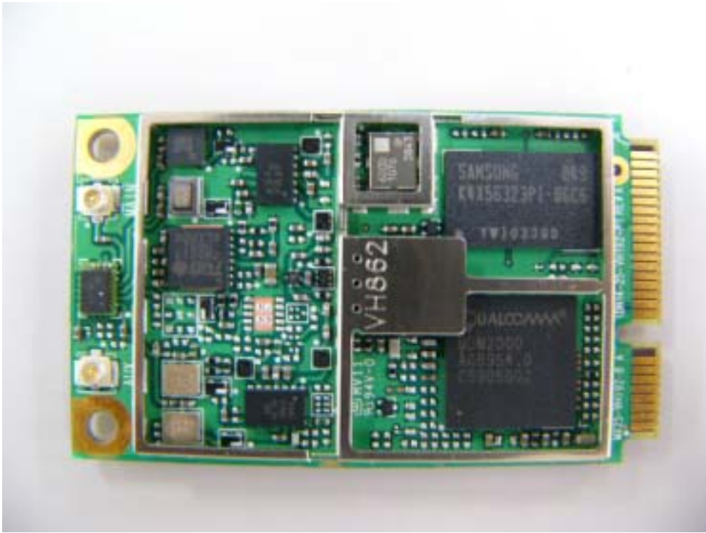
WWAN Module Interior Top View
