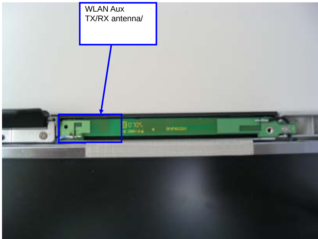
WLAN Aux antenna magnified view
