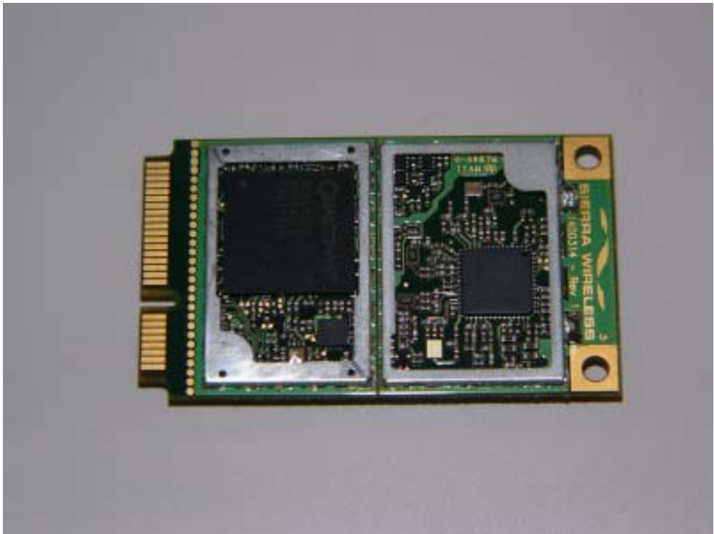
WWAN Module Interior Bottom View
