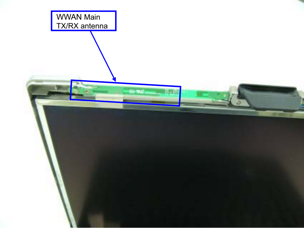
WWAN Main TX/RX Antenna
