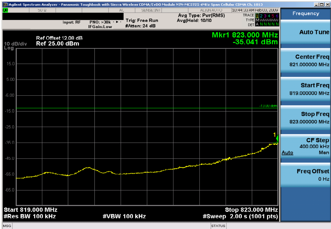
Plot 7-4. 4MHz Span Plot (Cellular CDMA Mode – Ch. 1013)
