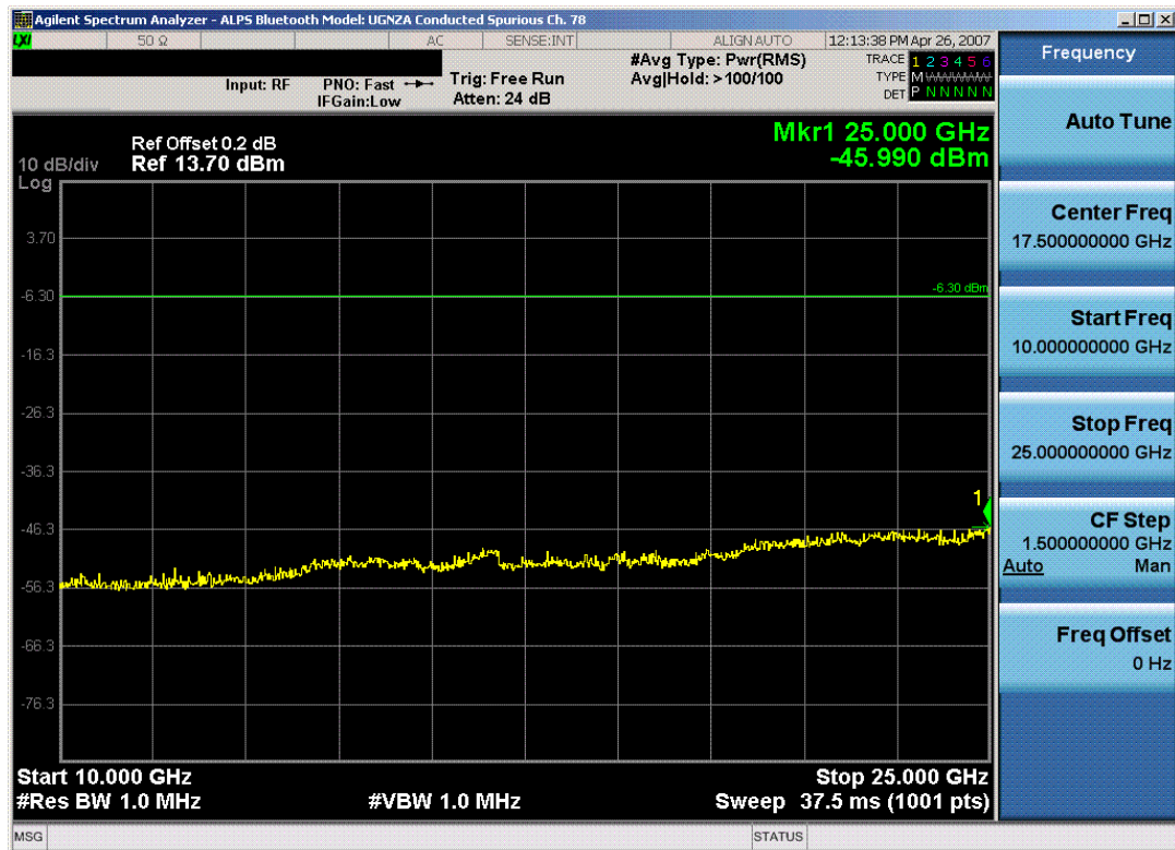
Plot 6-17. Conducted Spurious Plot (Bluetooth – Ch. 78)
