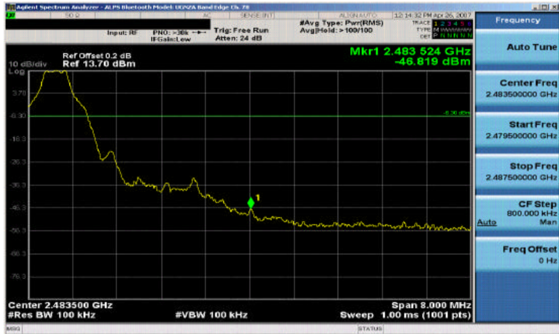
Plot 6-5. Band Edge Plot (Bluetooth – Ch. 78)
