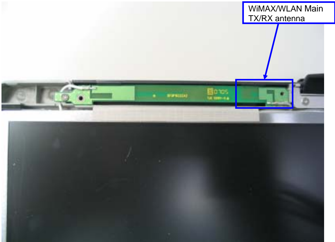
WiMAX/WLAN Main antenna magnified view
