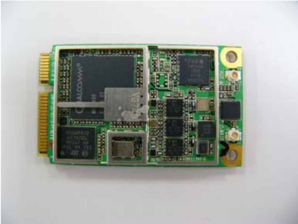
WWAN Module Interior Top View
