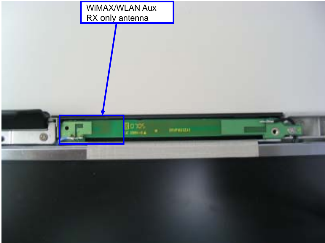
WiMAX/WLAN Aux antenna magnified view
