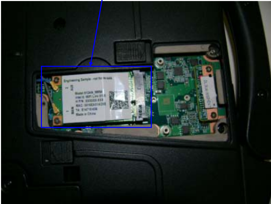
WiMAX/WLAN Module Magnified View
