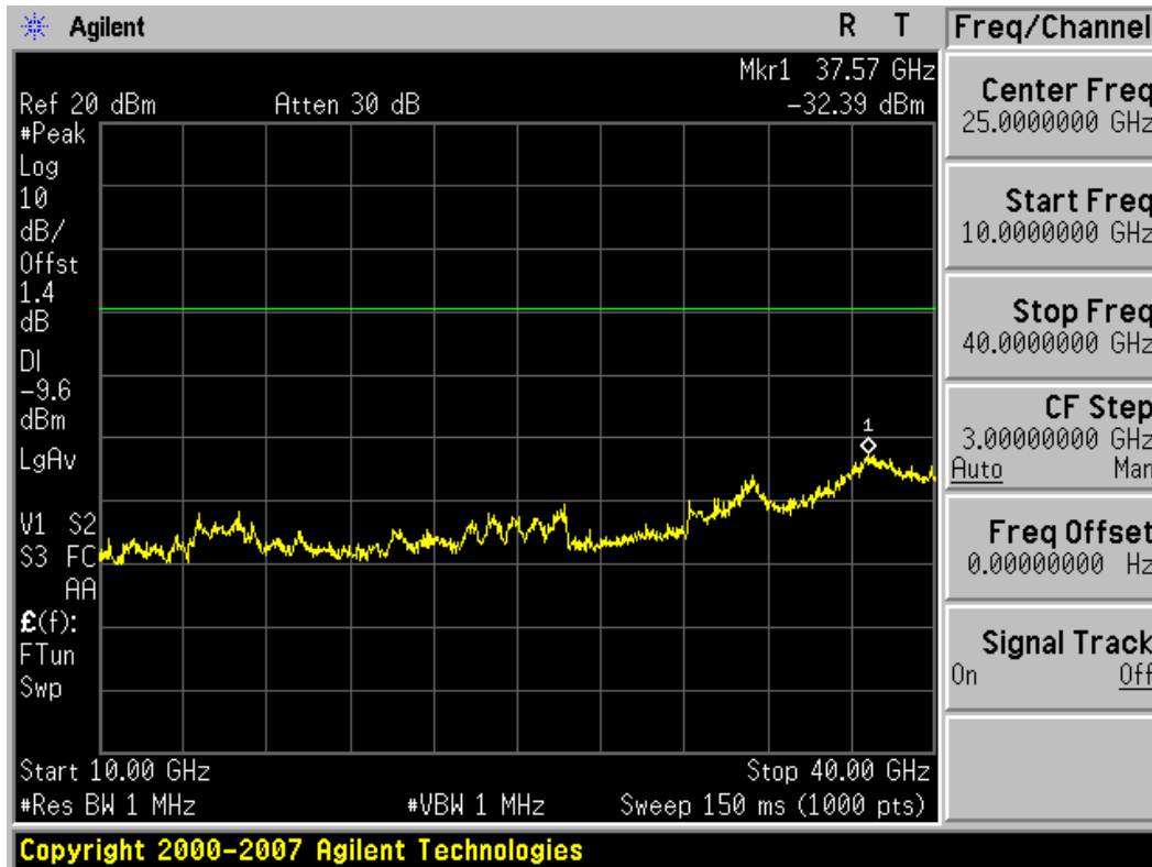
Plot 6-50. Conducted Spurious Plot (802.11a – Ch. 165)
