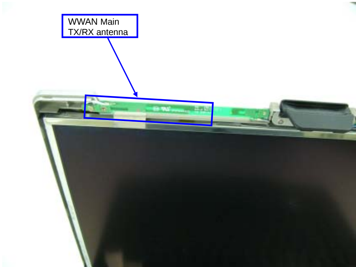
WWAN Main TX/RX Antenna
