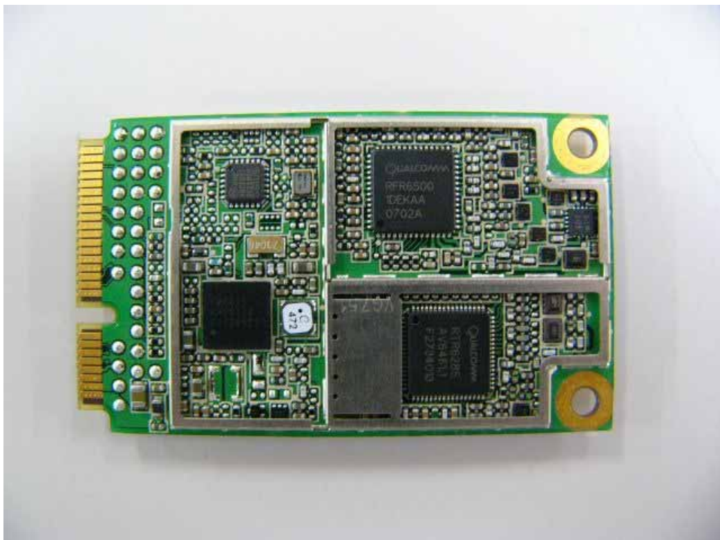
WWAN Module Interior Bottom View
