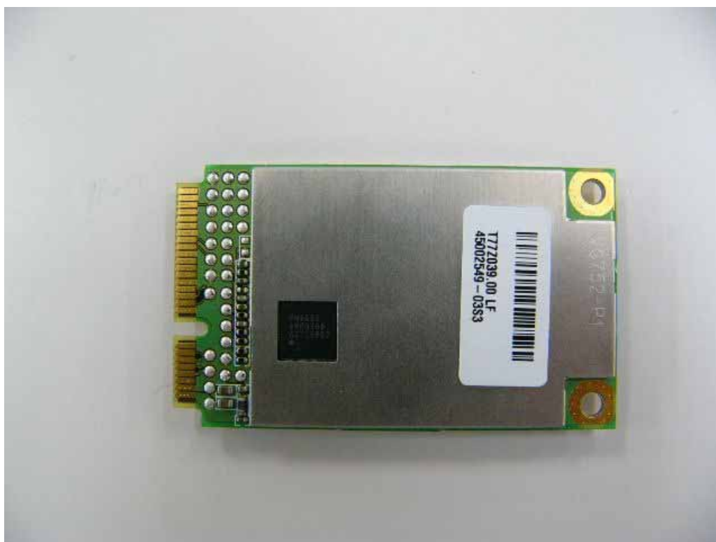
WWAN module Bottom View
