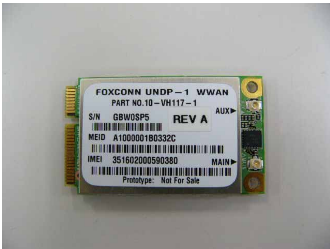
WWAN Module Top View
