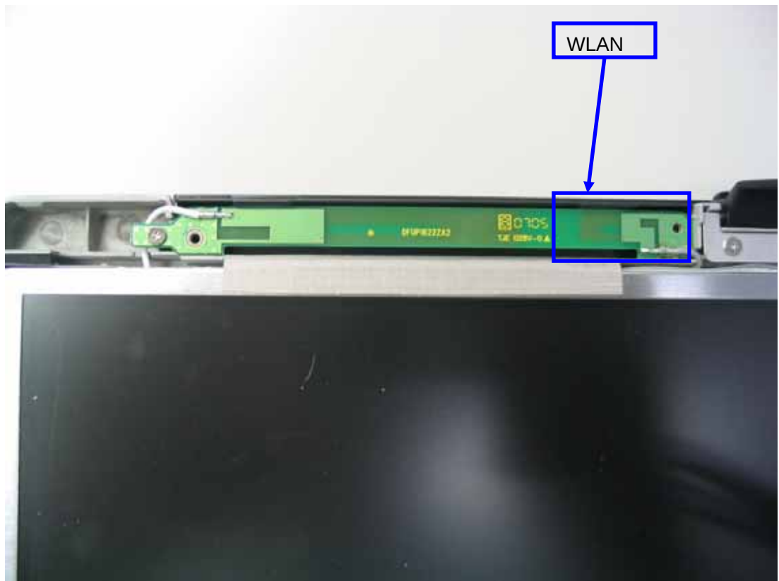
WLAN Main antenna magnified view
