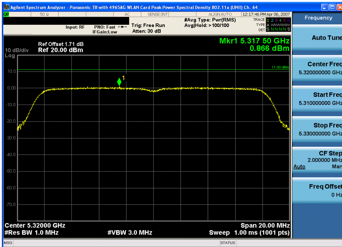
Plot 6-8. Peak Power Spectral Density Plot (802.11a (UNII) – Ch. 64)
