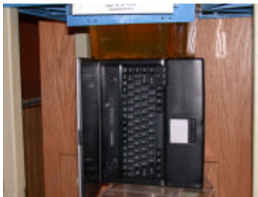
Figure 12.2.1 Body SAR - Main Antenna Bystander Position
