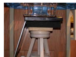
Figure 14.2 Body SAR Lap Position Test Setup
