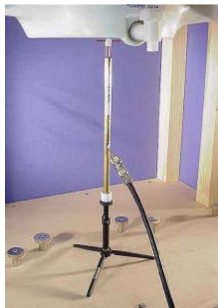
2450MHz System Performance Check Setup
