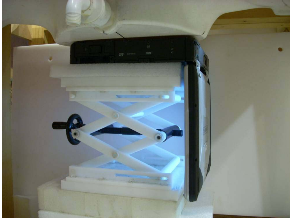
Figure 19-1 SAR Test Setup Photo 1 (Lap Position )
