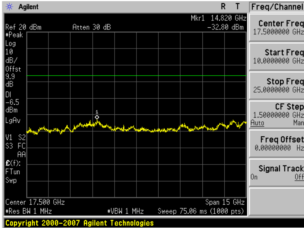
Plot 6-50. Conducted Spurious Plot (802.11b – Ch. 6) – Main Antenna
