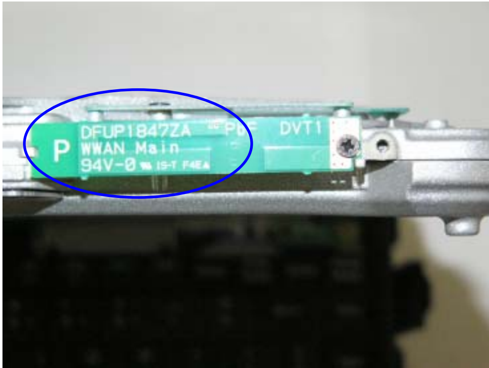
WWAN Main TX/RX Antenna
