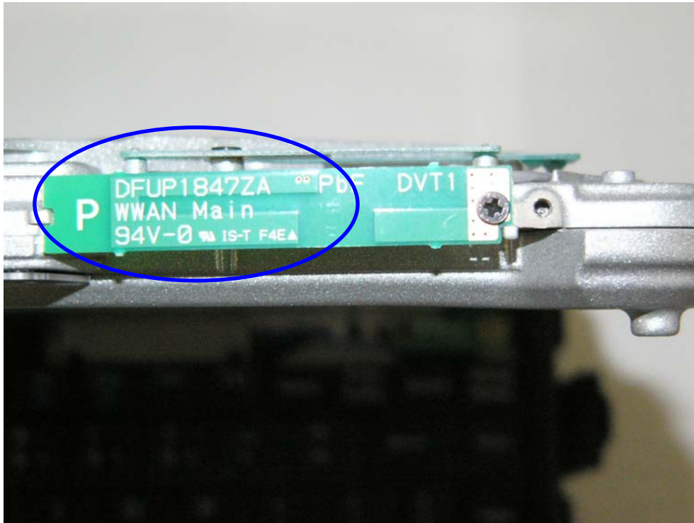
WWAN Main TX/RX Antenna
