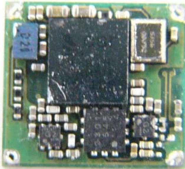
Bluetooth Module inside Top View
