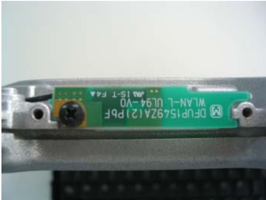
WLAN Main TX/RX Antenna
