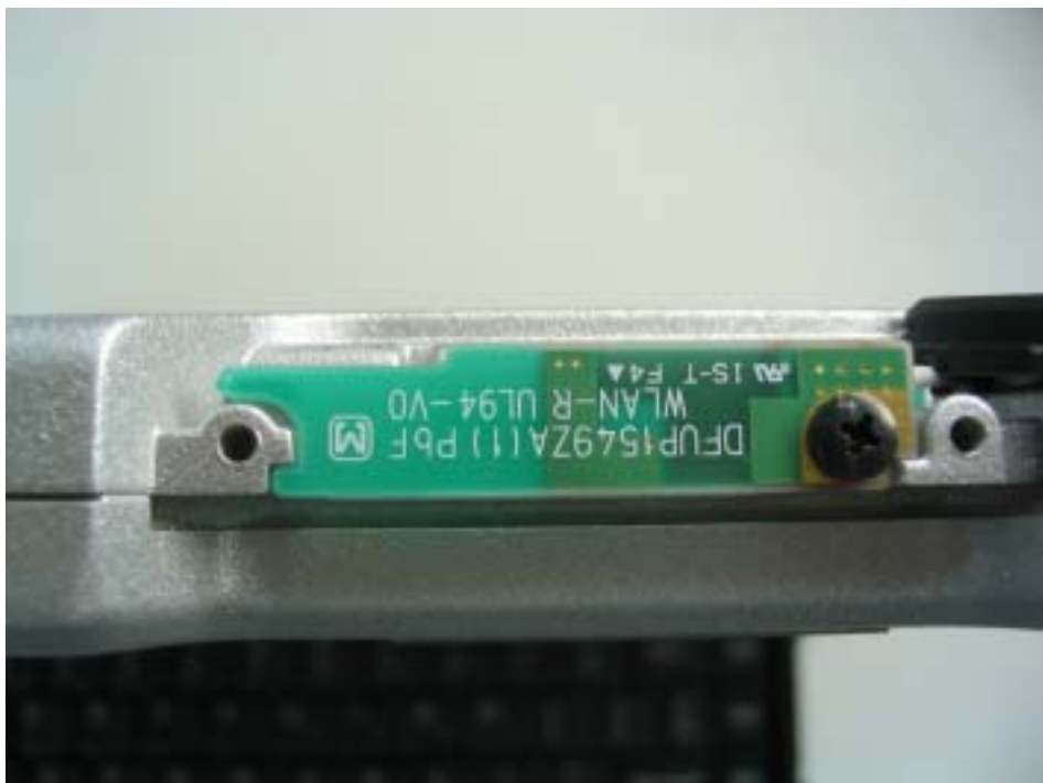
WLAN Aux TX/RX Antenna
