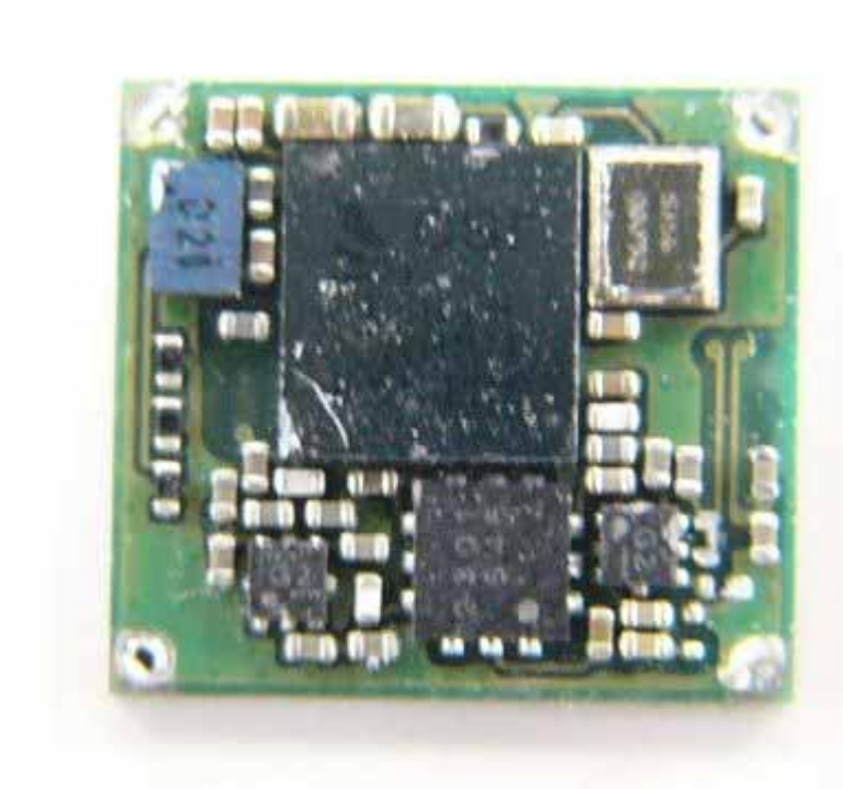
Bluetooth Module inside Top View
