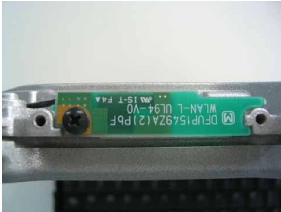
WLAN Main TX/RX Antenna
