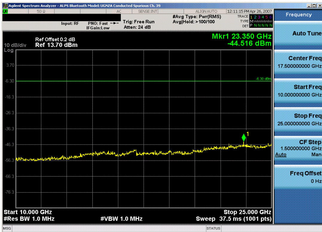
Plot 6-15. Conducted Spurious Plot (Bluetooth – Ch. 39)
