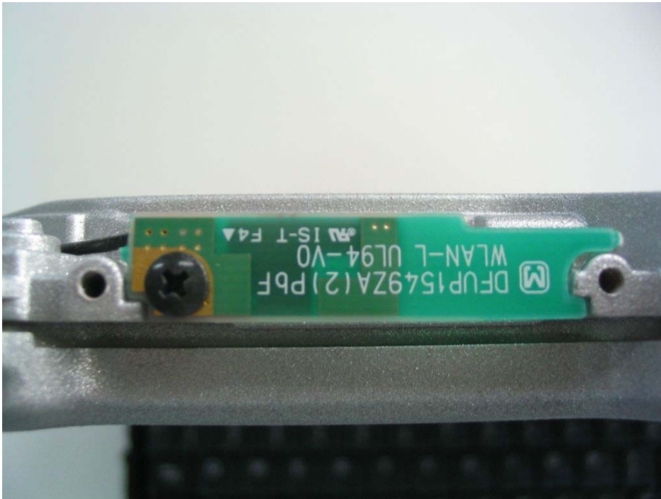
WLAN Main TX/RX Antenna
