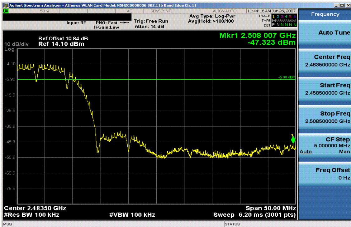
Plot 6-14. Band Edge Plot (802.11b – Ch. 11)
