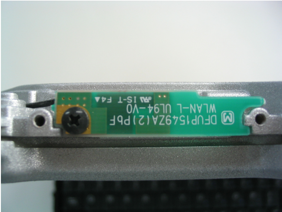
WLAN Main TX/RX Antenna
