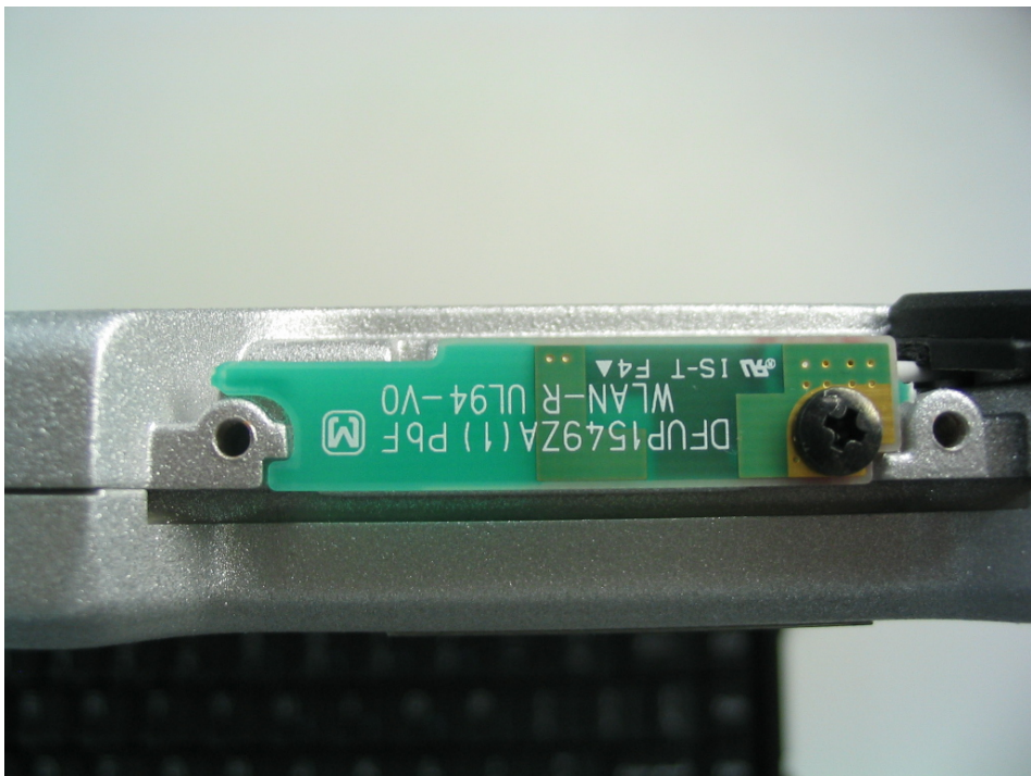
WLAN AUX TX/RX Antenna
