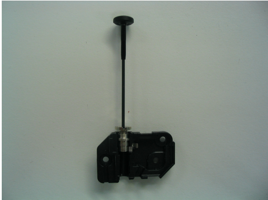
HSDPA Main TX/RX Antenna
