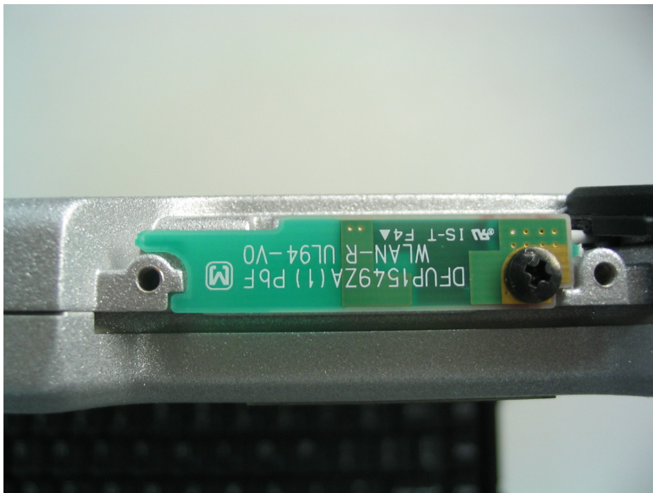
WLAN AUX TX/RX Antenna
