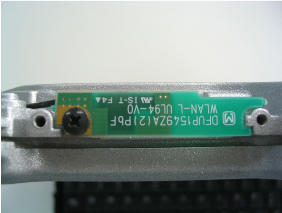
WLAN Main TX/RX Antenna
