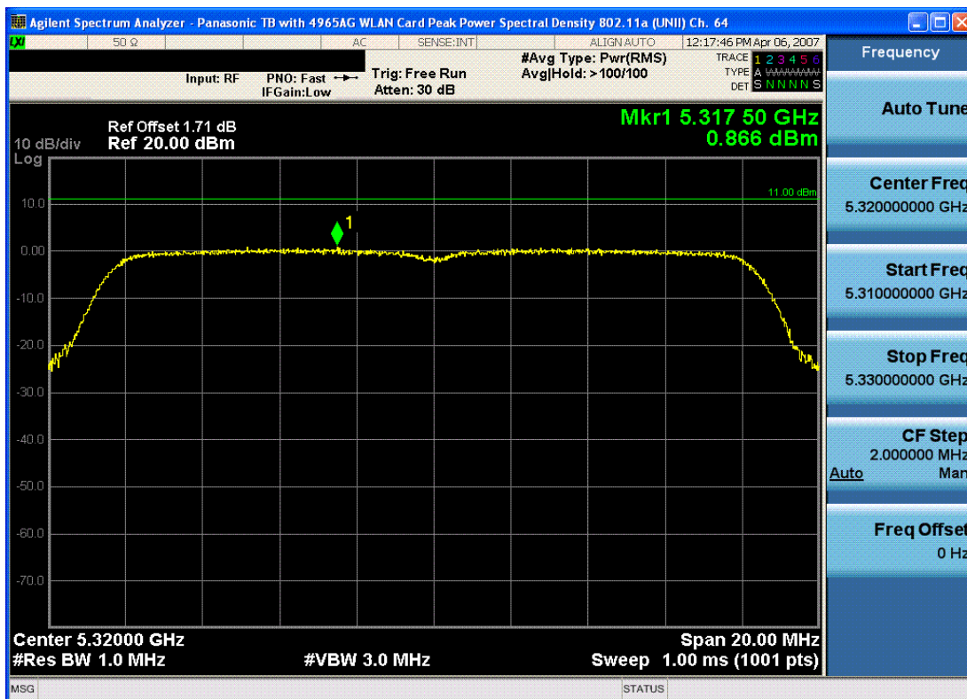
Plot 6-7. Peak Power Spectral Density Plot [FCC / IC] (802.11a (UNII) – Ch. 64)
