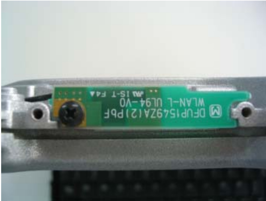
WLAN Main TX/RX Antenna
