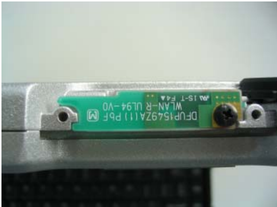
WLAN AUX TX/RX Antenna
