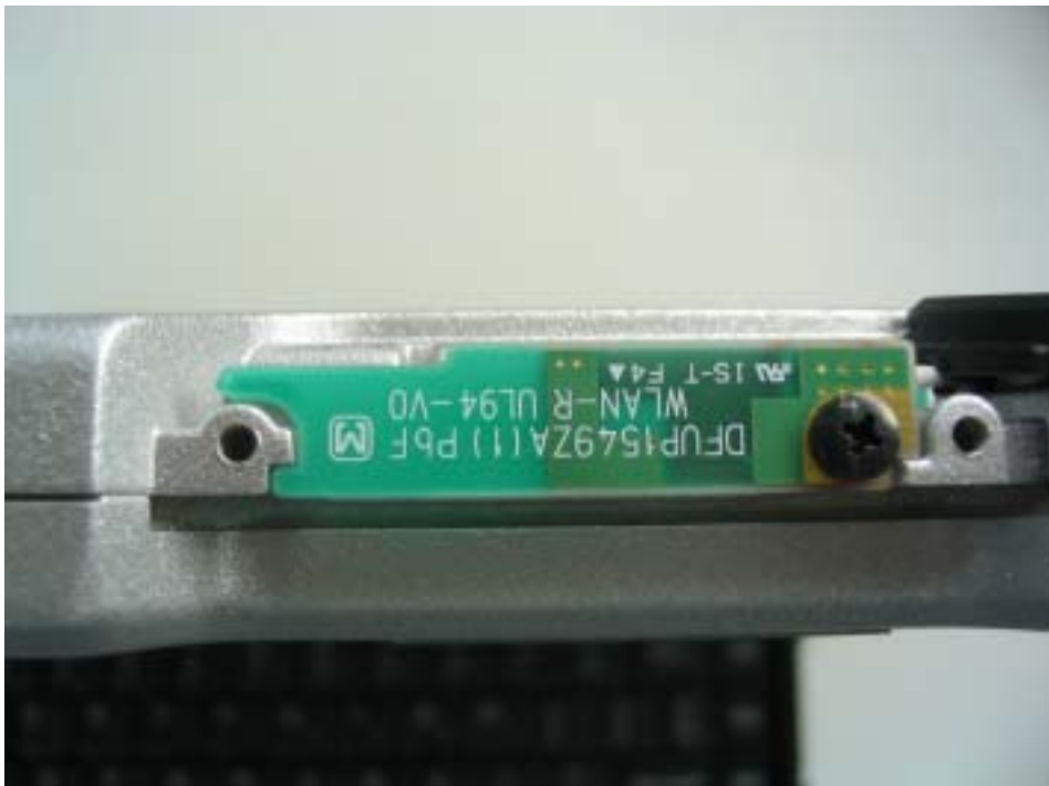
WLAN AUX TX/RX Antenna
