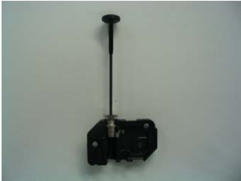
HSDPA Main TX/RX Antenna
