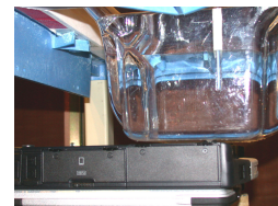
Figure 12.2 Body SAR - Lap Position -
