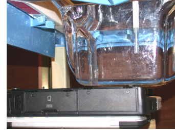
Figure 7.1 Body SAR Laptop Configuration
