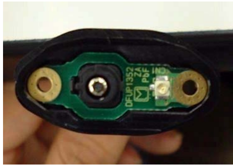
HSDPA TXRX Antenna I/F PWB
