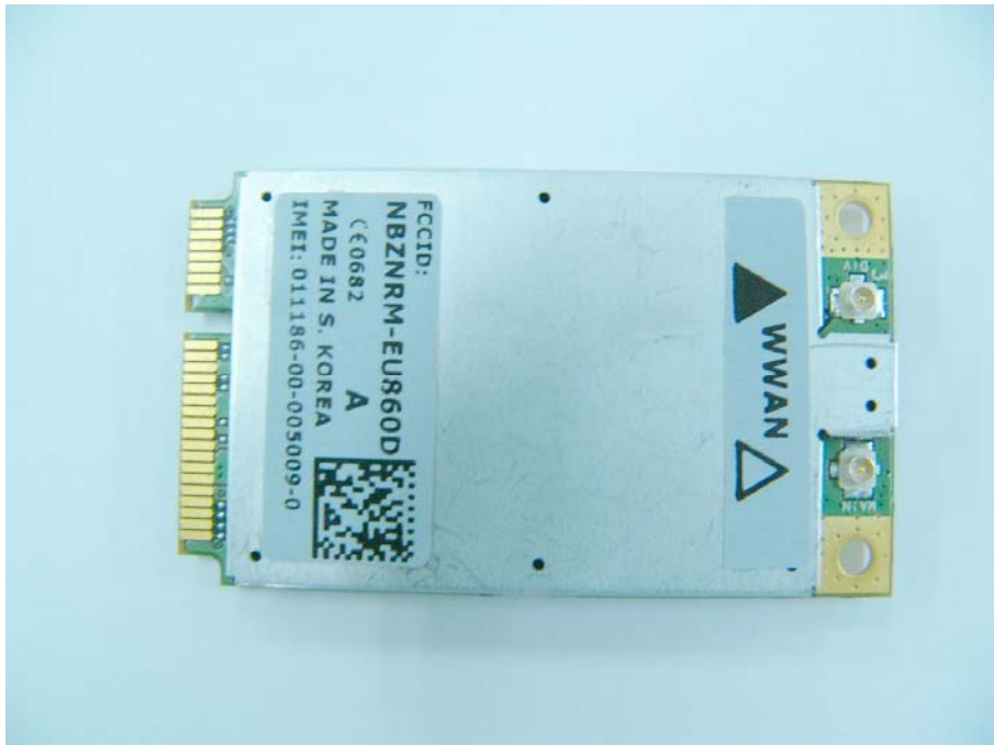
HSDPA Module Top View
