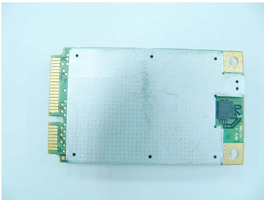
HSDPA Module Bottom View
