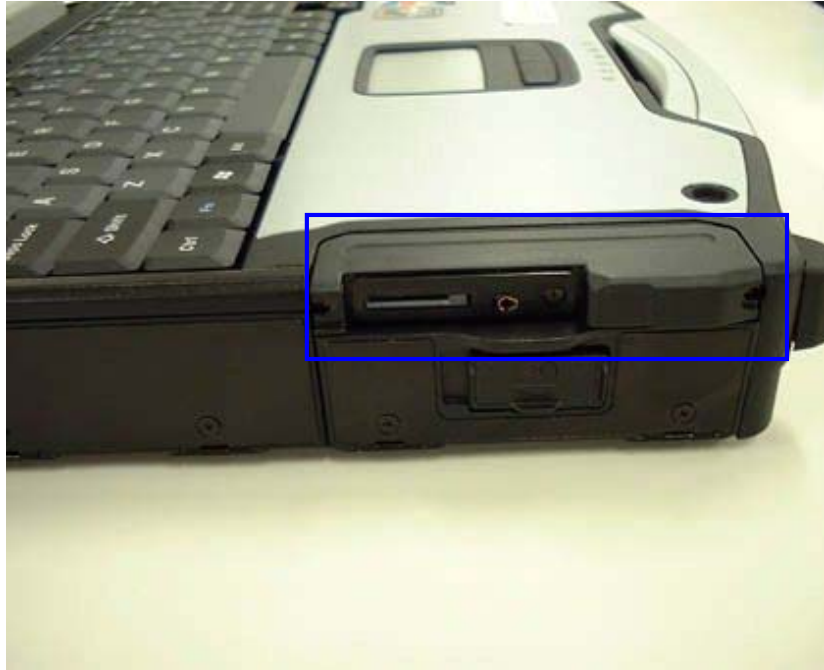
HSDPA Module Adapter Position
