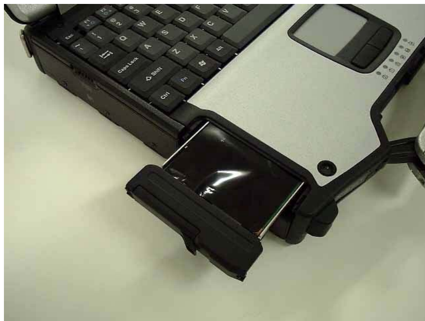
HSDPA Module Pack Slide Position
