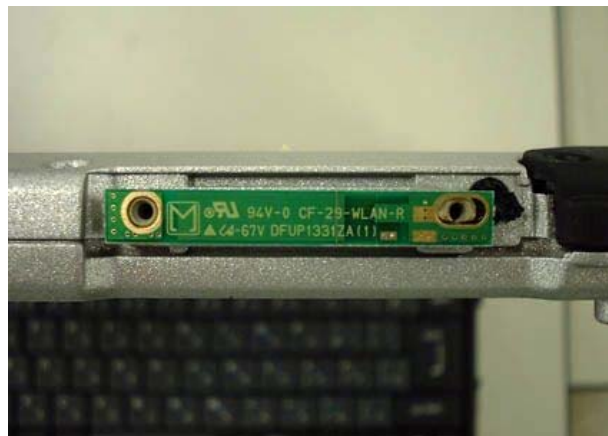
WLAN Main TX/RX Antenna View
