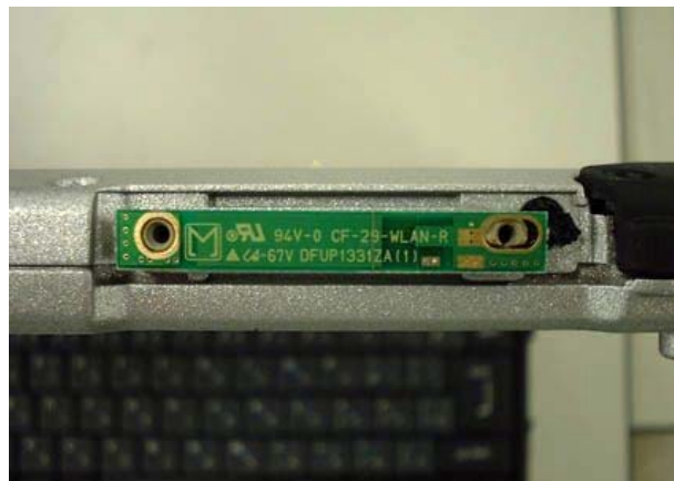
WLAN Main TX/RX Antenna View
