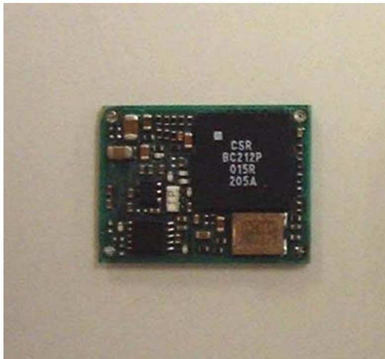
Bluetooth Module without shield
