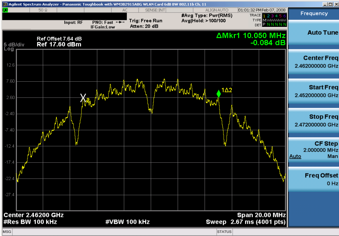
Plot 6-3. 6dB Bandwidth Plot (802.11b – Ch. 11)
