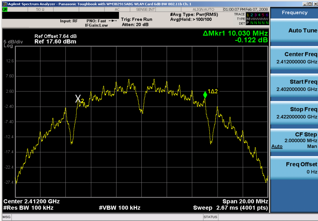
Plot 6-1. 6dB Bandwidth Plot (802.11b – Ch. 1)
