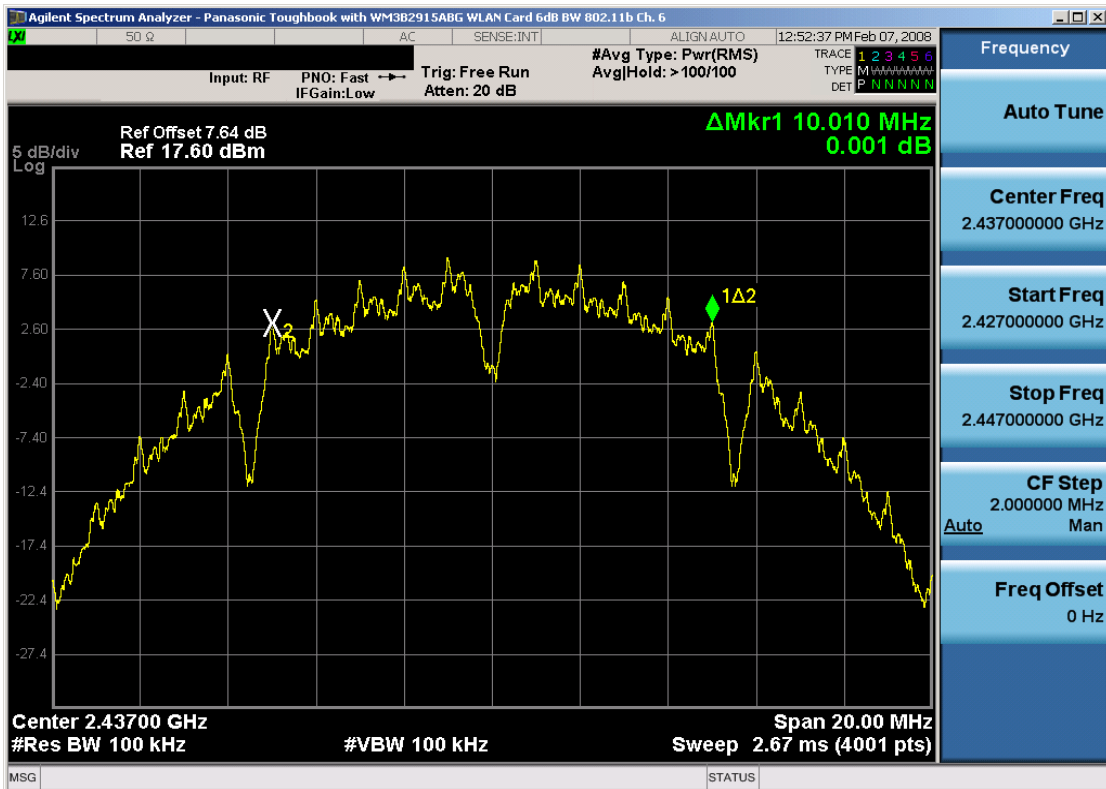
Plot 6-2. 6dB Bandwidth Plot (802.11b – Ch. 6)
