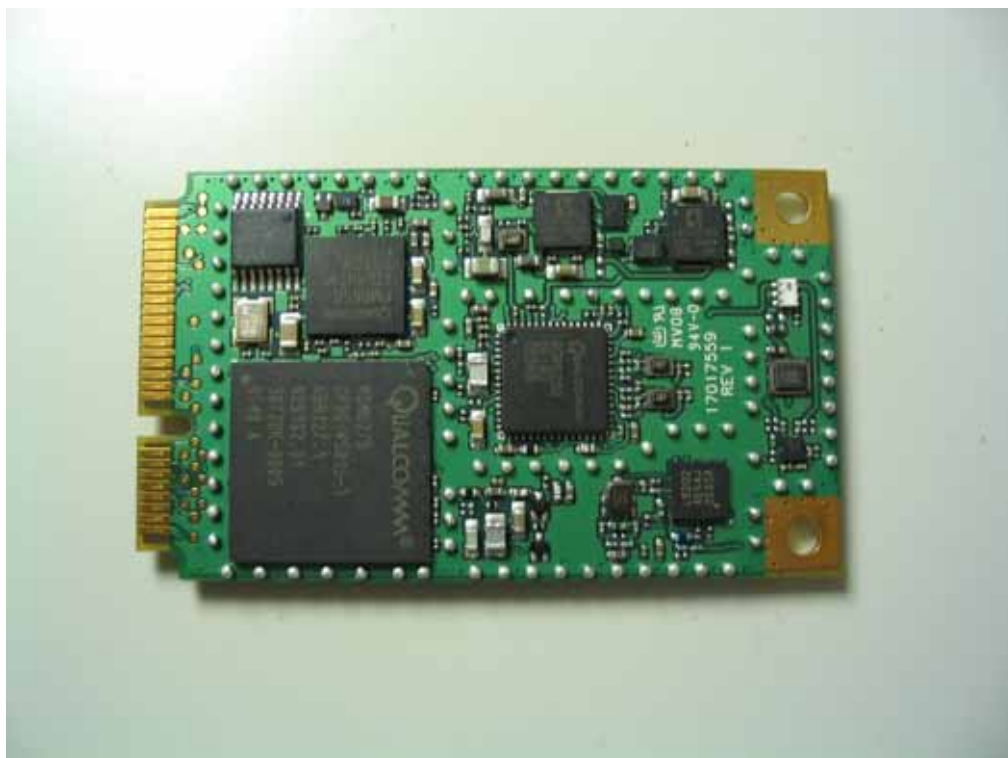
HSDPA Module Interior Bottom View
