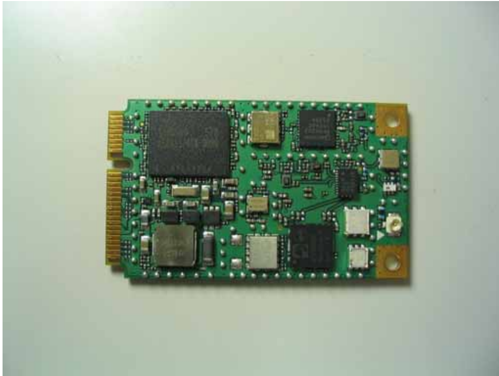
HSDPA Module Interior Top View
