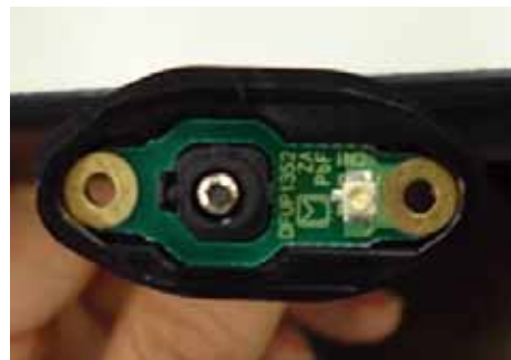
Whip Antenna I/F PCB
