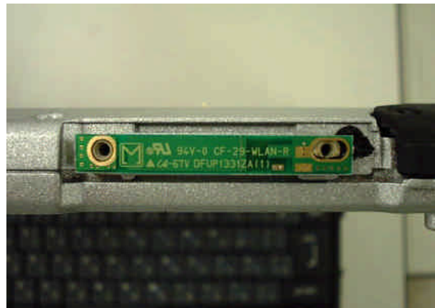
Send & Receive Antenna View
