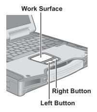
Use the touch pad to move the cursor on the display and perform normal computer operations. For instructions on how to operate, refer to Reference "Touch Pad".
