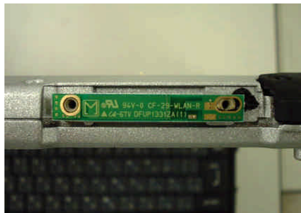
Send & Receive Antenna View
