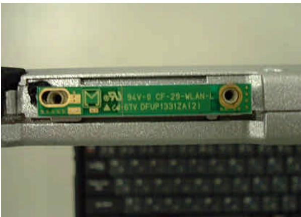
Receive only Antenna View
