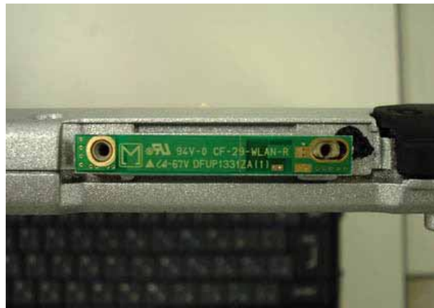
Main TX/RX Antenna View
