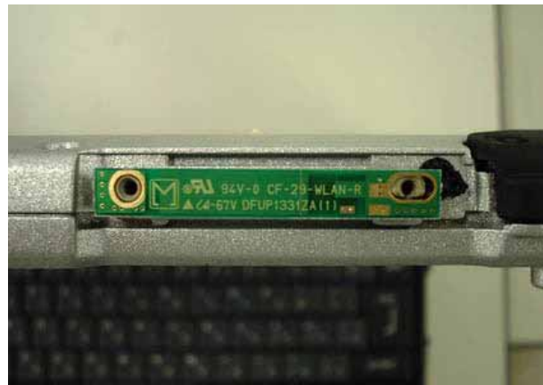
Main TX/RX Antenna View
