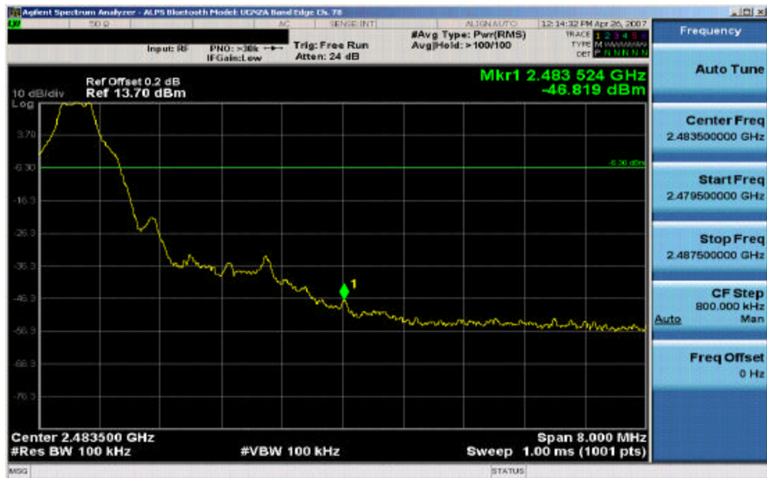
Plot 6-5. Band Edge Plot (Bluetooth – Ch. 78)
