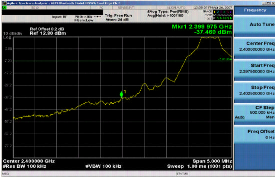
Plot 6-4. Band Edge Plot (Bluetooth – Ch. 0)
