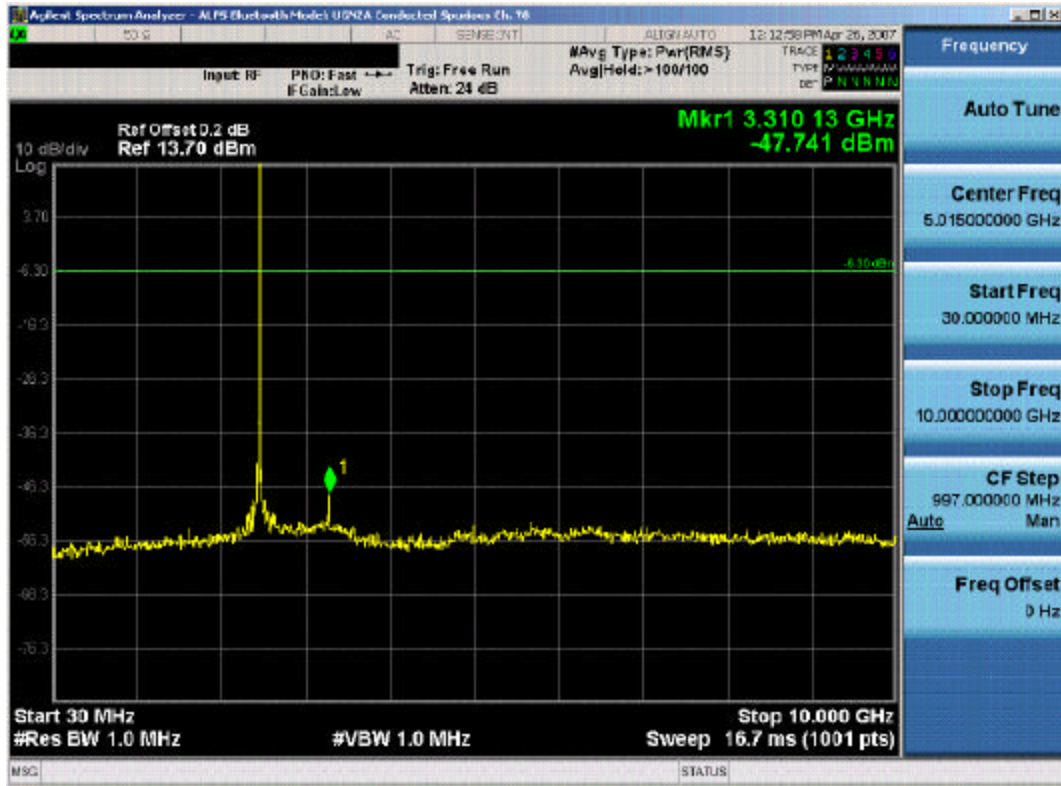
Plot 6-16. Conducted Spurious Plot (Bluetooth – Ch. 78)
