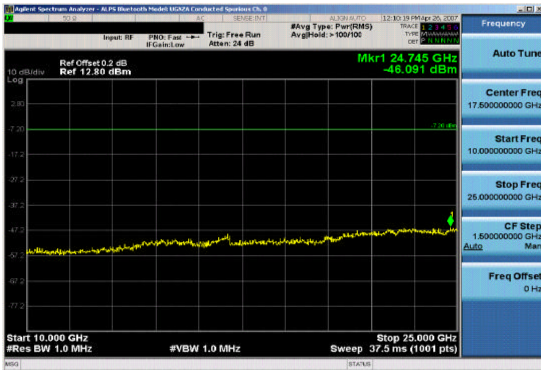
Plot 6-13. Conducted Spurious Plot (Bluetooth – Ch. 0)
