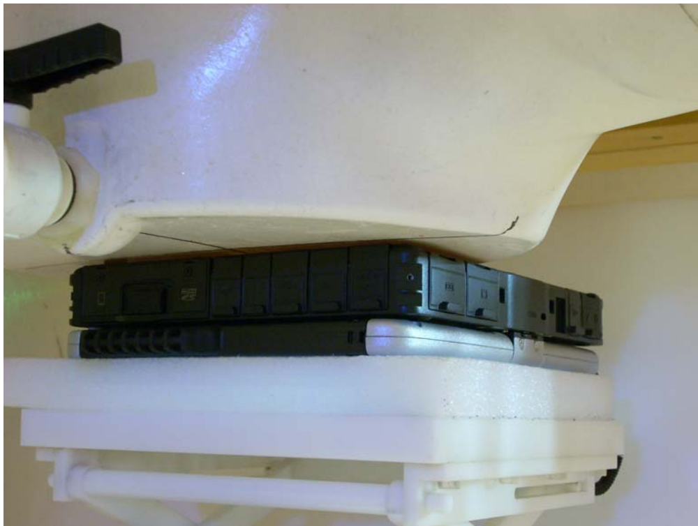
Figure 19-6 SAR Test Setup Photo 6 (Laptop Right Side)
