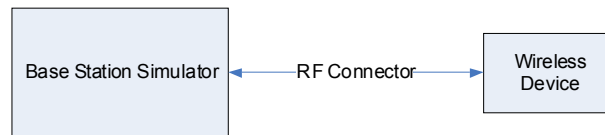
Figure 13-1 Power Measurement Setup
