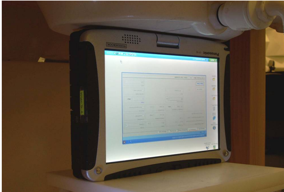
Figure 19-1 SAR Test Setup Photo 1 (Tablet Bottom)
