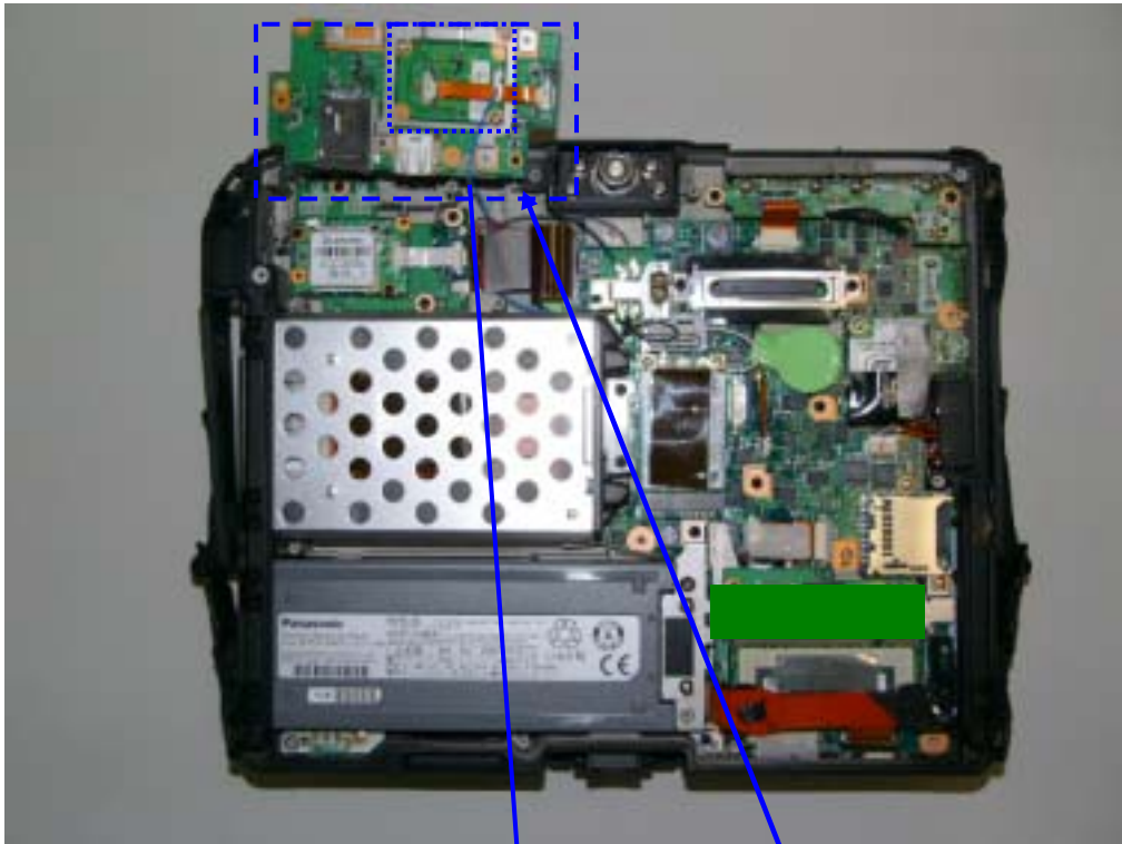
Reverse side of RF PWB
