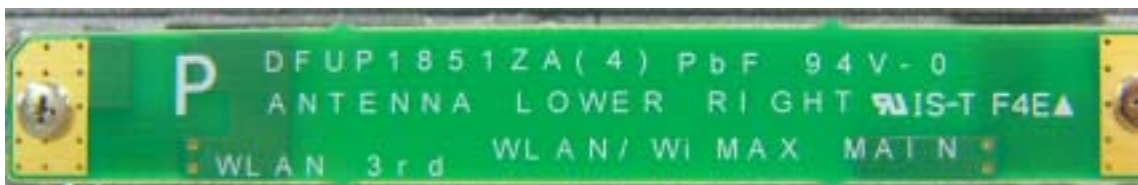
WLAN Main TX/RX Antenna
