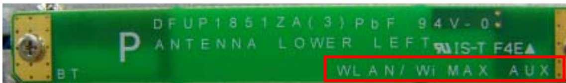
WLAN Aux TX/RX Antenna
