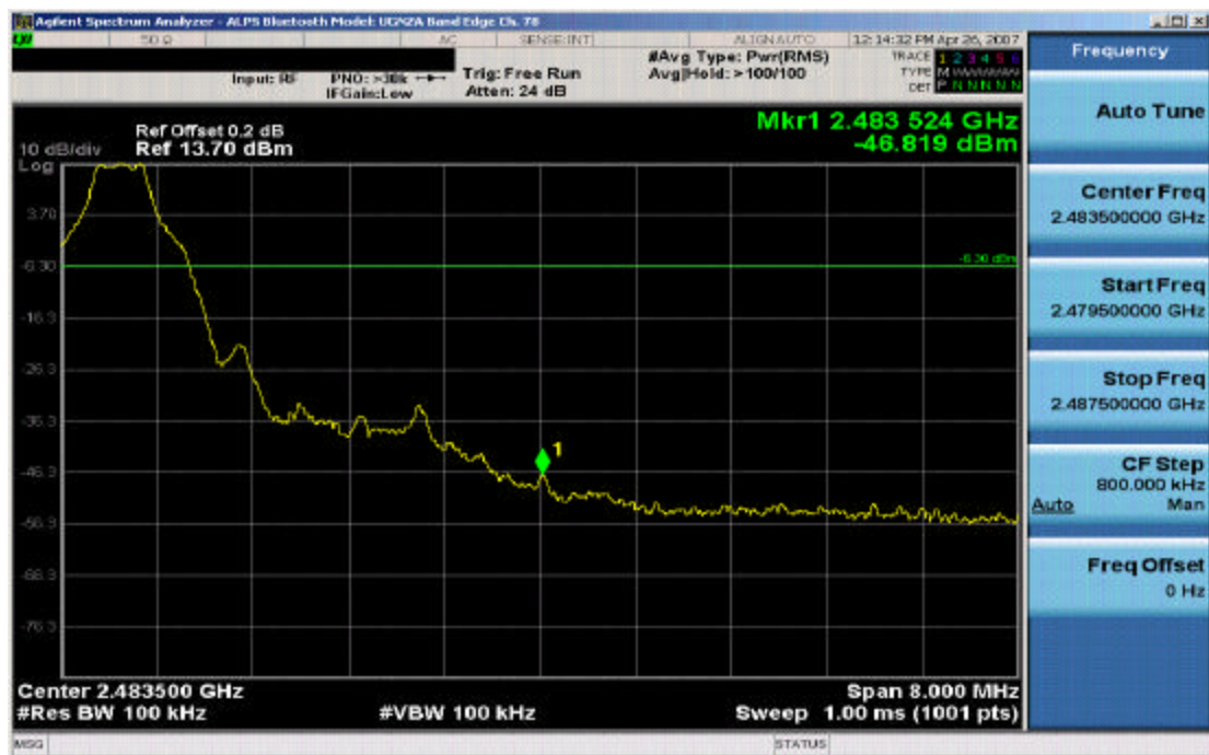
Plot 6-5. Band Edge Plot (Bluetooth – Ch. 78)
