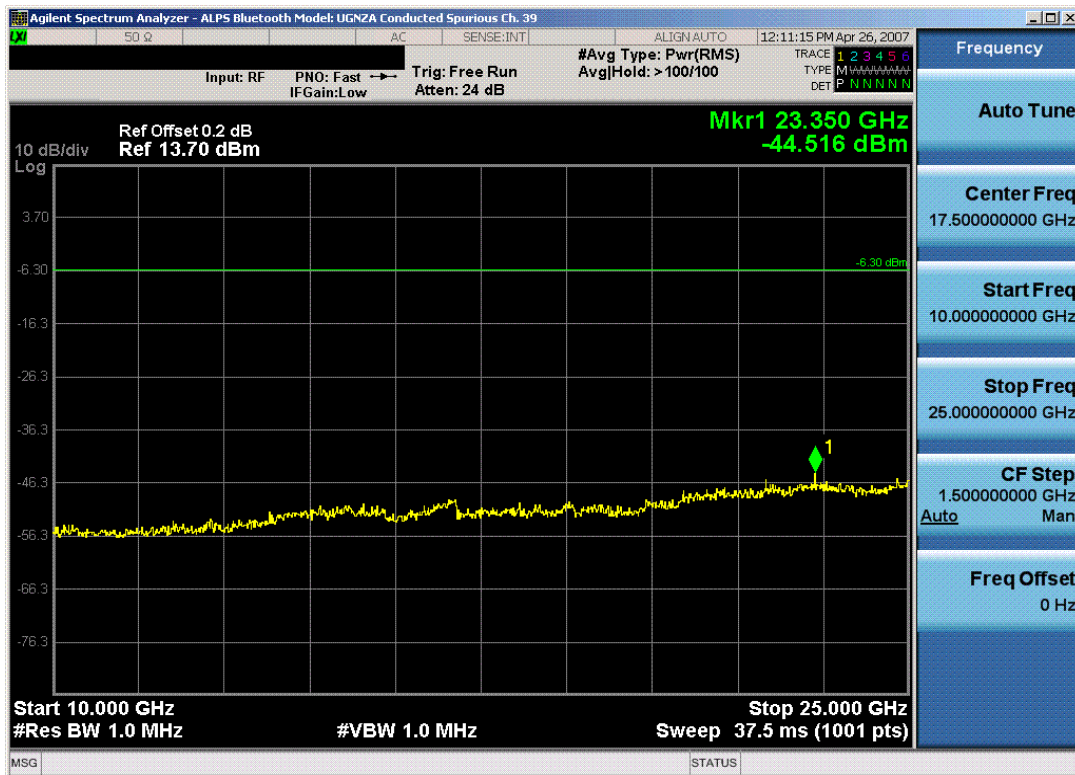
Plot 6-15. Conducted Spurious Plot (Bluetooth – Ch. 39)
