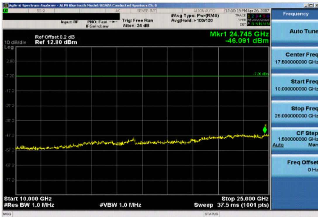
Plot 6-13. Conducted Spurious Plot (Bluetooth – Ch. 0)
