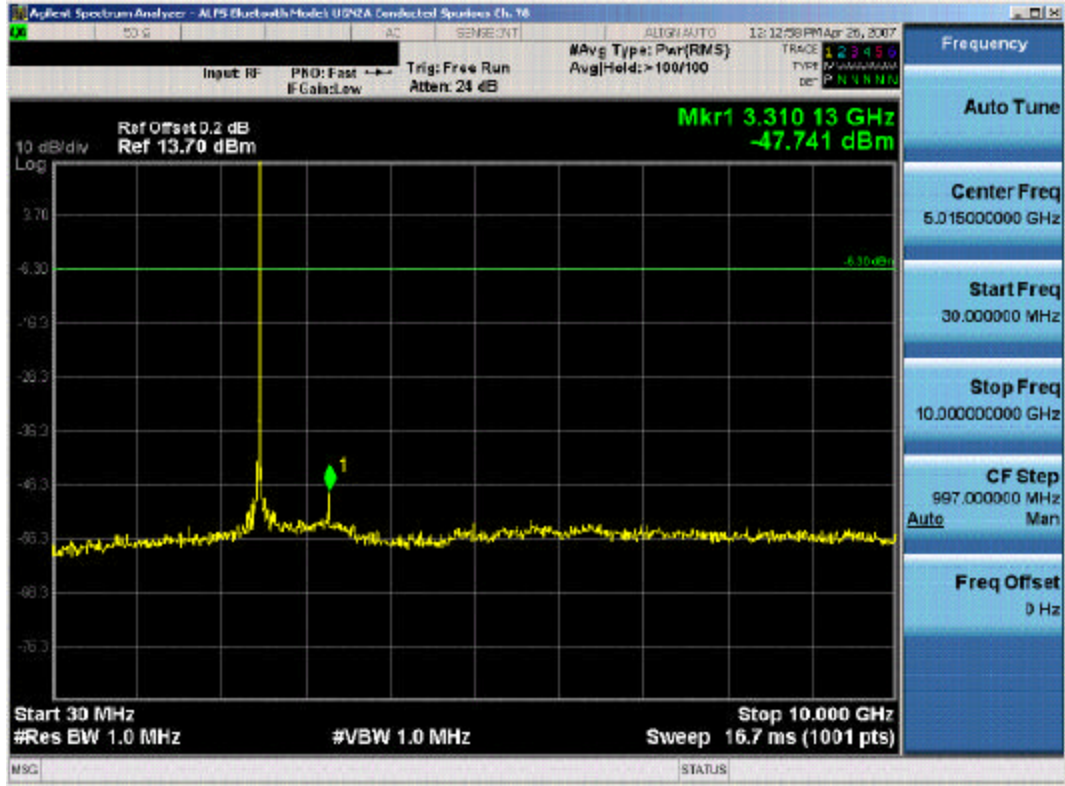
Plot 6-16. Conducted Spurious Plot (Bluetooth – Ch. 78)
