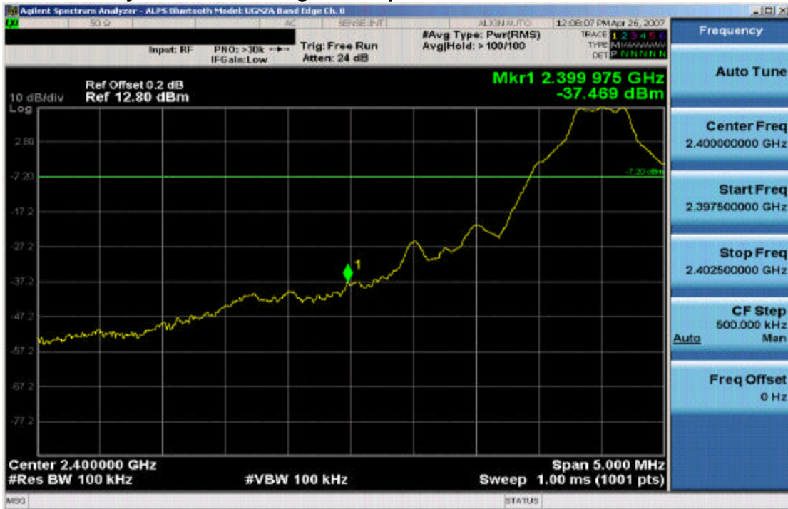
Plot 6-4. Band Edge Plot (Bluetooth – Ch. 0)
