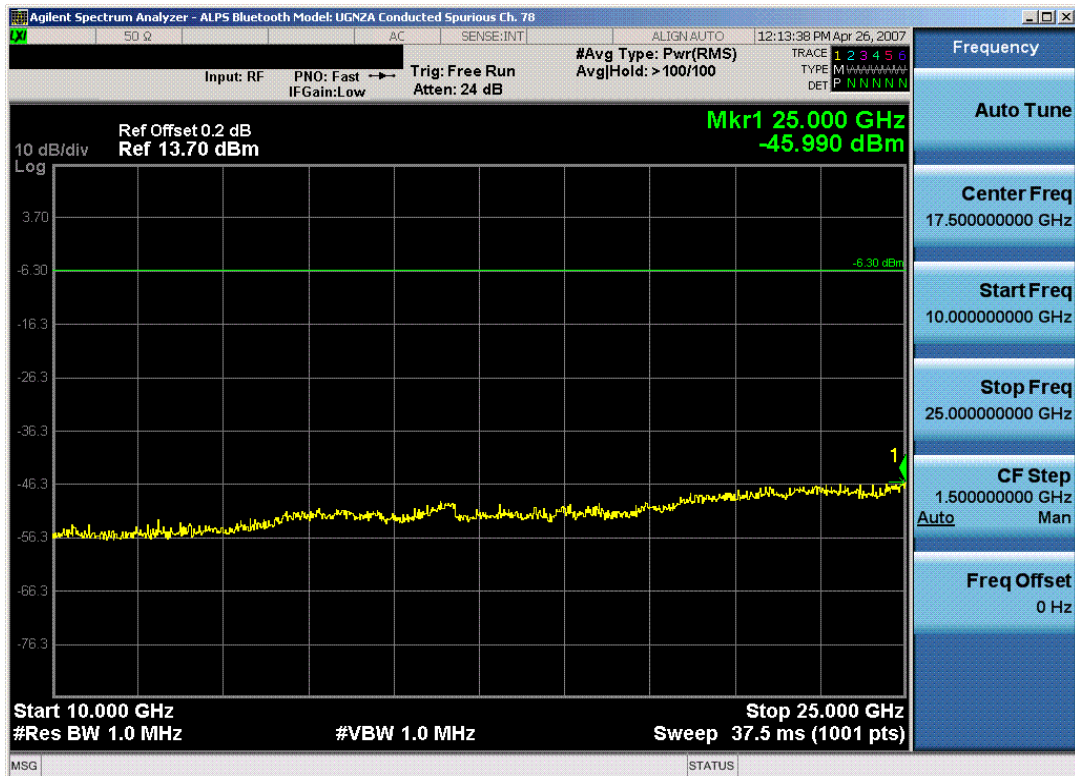
Plot 6-17. Conducted Spurious Plot (Bluetooth – Ch. 78)
